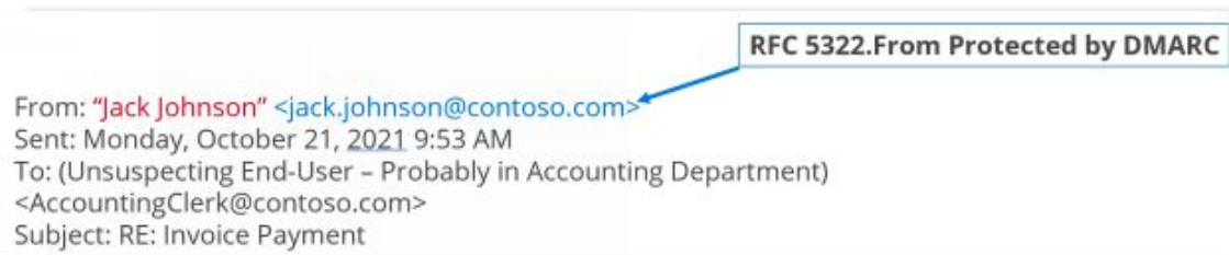
Figure 11 The RFC5322.From address is used by modern email clients (since 2008), not the RFC5321.From Envelope address
