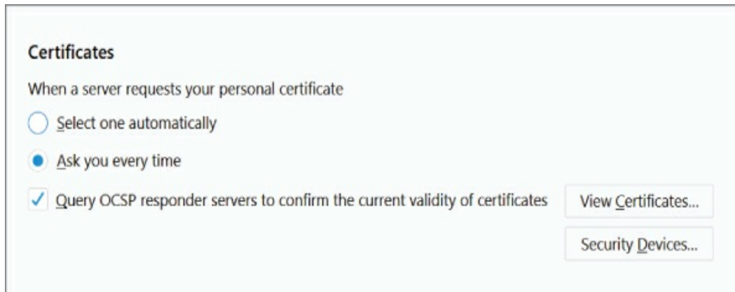
Figure 11.14: Loading the CA certificate into Firefox Preferences located under Privacy And Security
