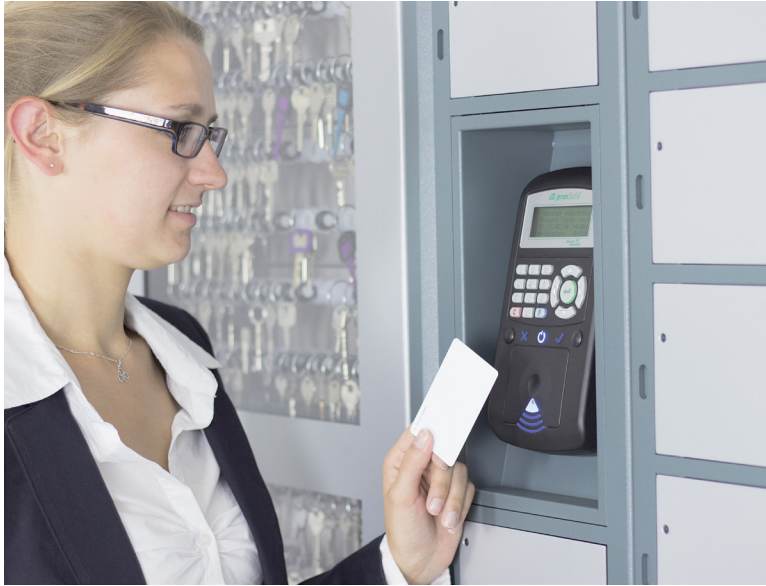
FIGURE 10.2 Linking key control with an electronic system. Management of physical keys, as seen here, or weapons or other physical assets can be controlled with an RFID-enabled access. Removal and return of keys, or other assets, are both recorded and linked to the person accessing the cabinet. (Source: Deister Electronics USA.)
