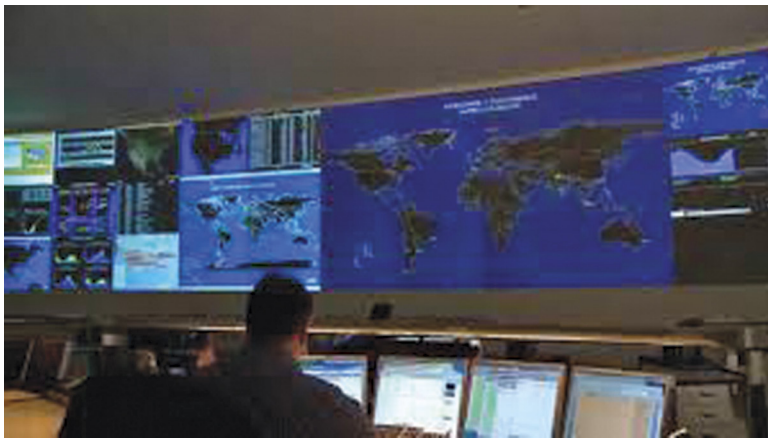
FIGURE 10.4 Communications and command in a control center. Internet protocol television (IPTV) and closed-circuit television (CCTV) are integral parts of a comprehensive premises protection plan. Here a security monitor is able to view data and live action on displays. Action requiring greater attention can be switched to one of the large screens in the center. (Source: AT&T.)
