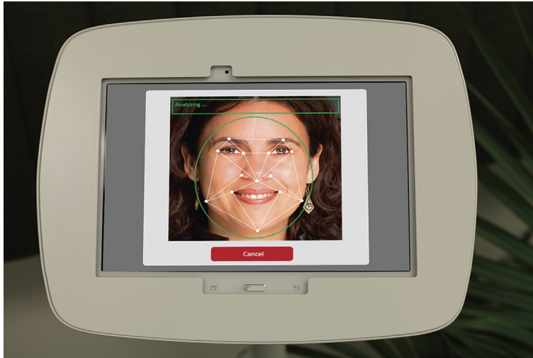
FIGURE 9.2 Using biometrics to coordinate with time and attendance. Workplaces are able to obtain time and attendance data remotely. This system uses facial recognition technology along with precise location services using GPS, IP addresses, and cellular triangulation to provide assurance that the security officer is reporting in where he or she is expected to be. Information collected from the worker's biometric input is the basis for time and labor management and payroll. (Source: Valiant Solutions.)
